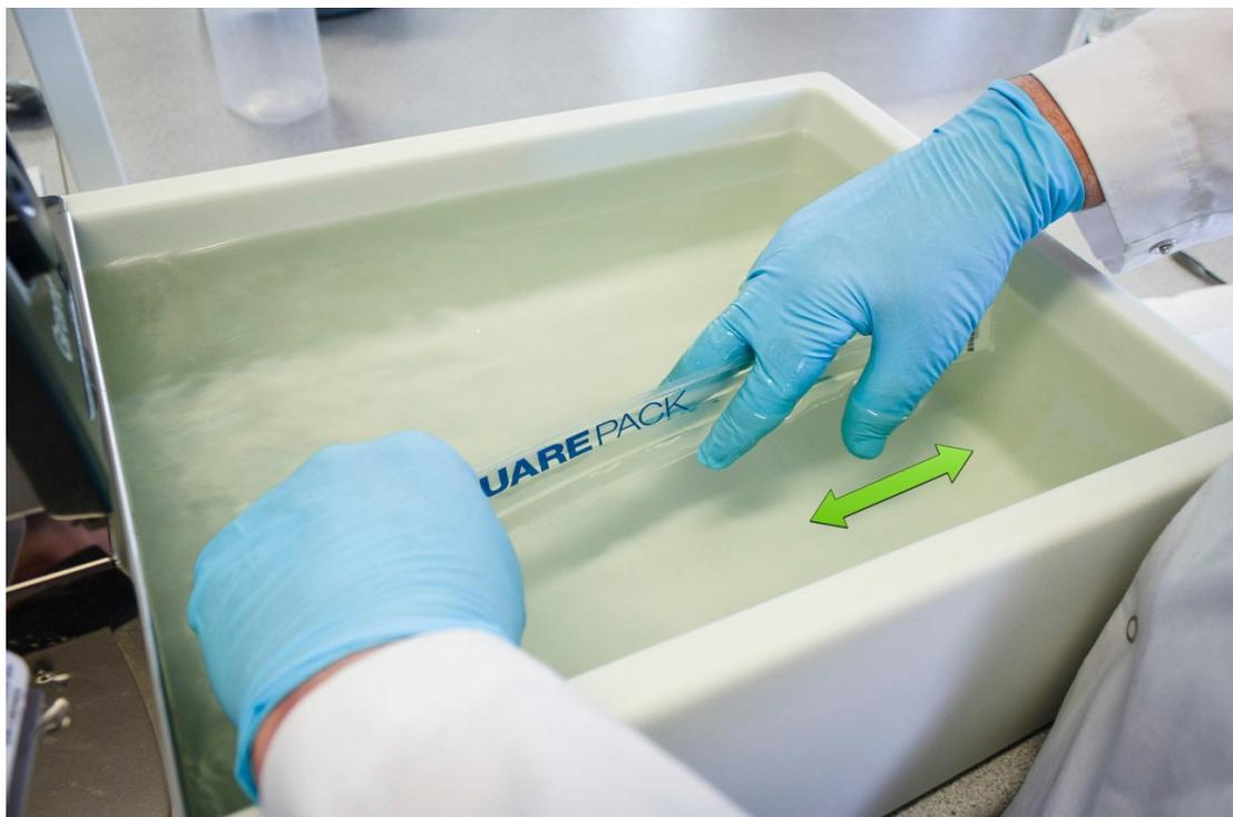
Figure 6 Thawing one Squarepack®. Move fingers in a lateral motion to ensure a correct thawing curve.
