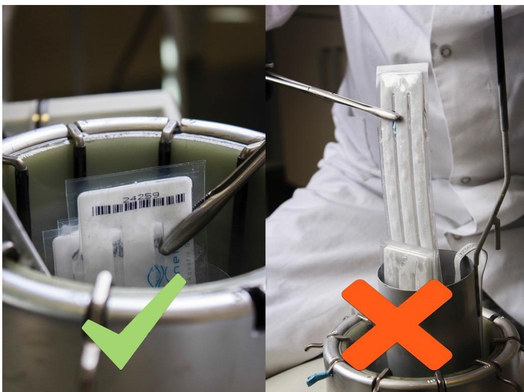
Figure 3 How to correctly handle and identify cryopreserved milt in Squarepacks<sup>®</sup> (left). Lifting Squarepacks<sup>®</sup> above the neck of the dewar (right) lead to partial thawing and could mean poor fertilization results.
