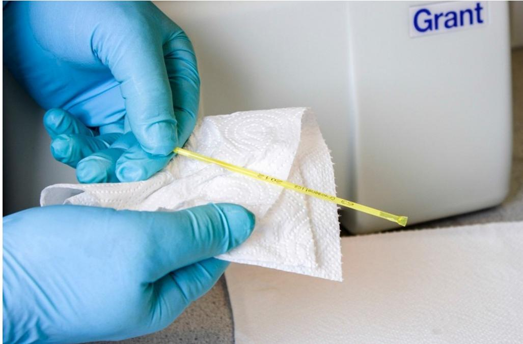
*Figure 9 It is important to dry the milt container well before opening.*
